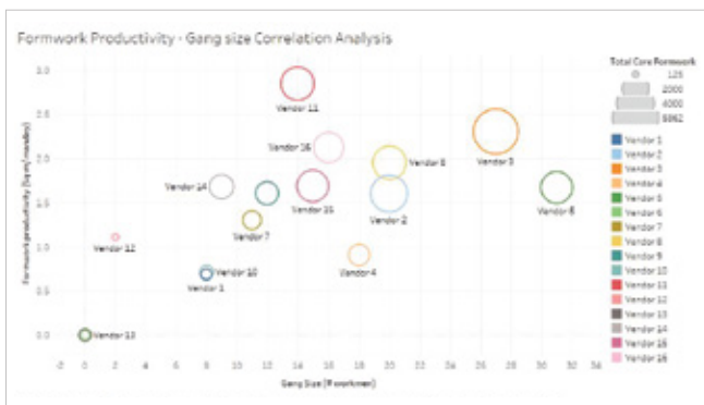
Figure 4: Analysis depicting correlation between gang size, productivity & quantity of work done by vendors
